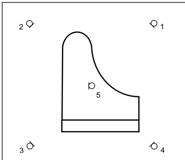
Figure 7: Positions of the five microphones for the recording of the piano.
