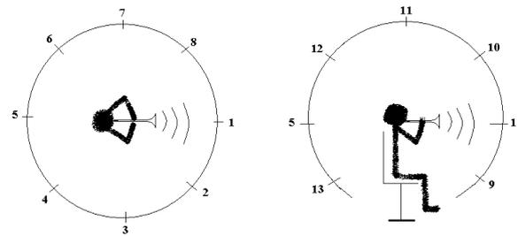
Figure 6: Positions of the 13 microphones for the recording of the clarinet. Only five of them are used here (no 1, 3, 5, 7, and 11).
