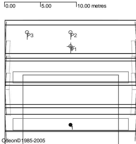
Figure 5: The three source positions and the receiver position. Only the front part of the concert hall is shown.
