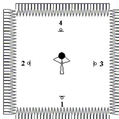
Figure 1: Anechoic recording with the multi-channel method, here shown with four microphones in the horizontal plane.
