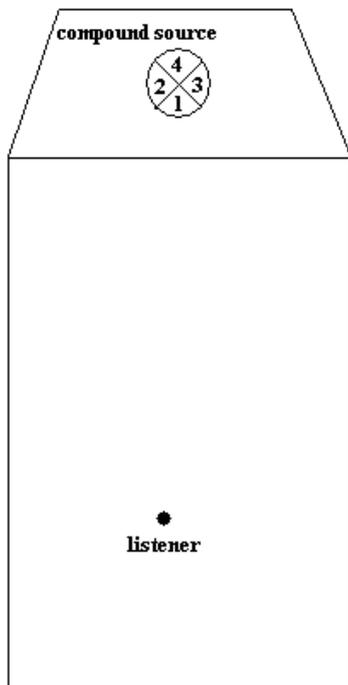
Figure 2: Room simulation with the multi-channel method. Each part of the compound source radiates into a solid angle.
