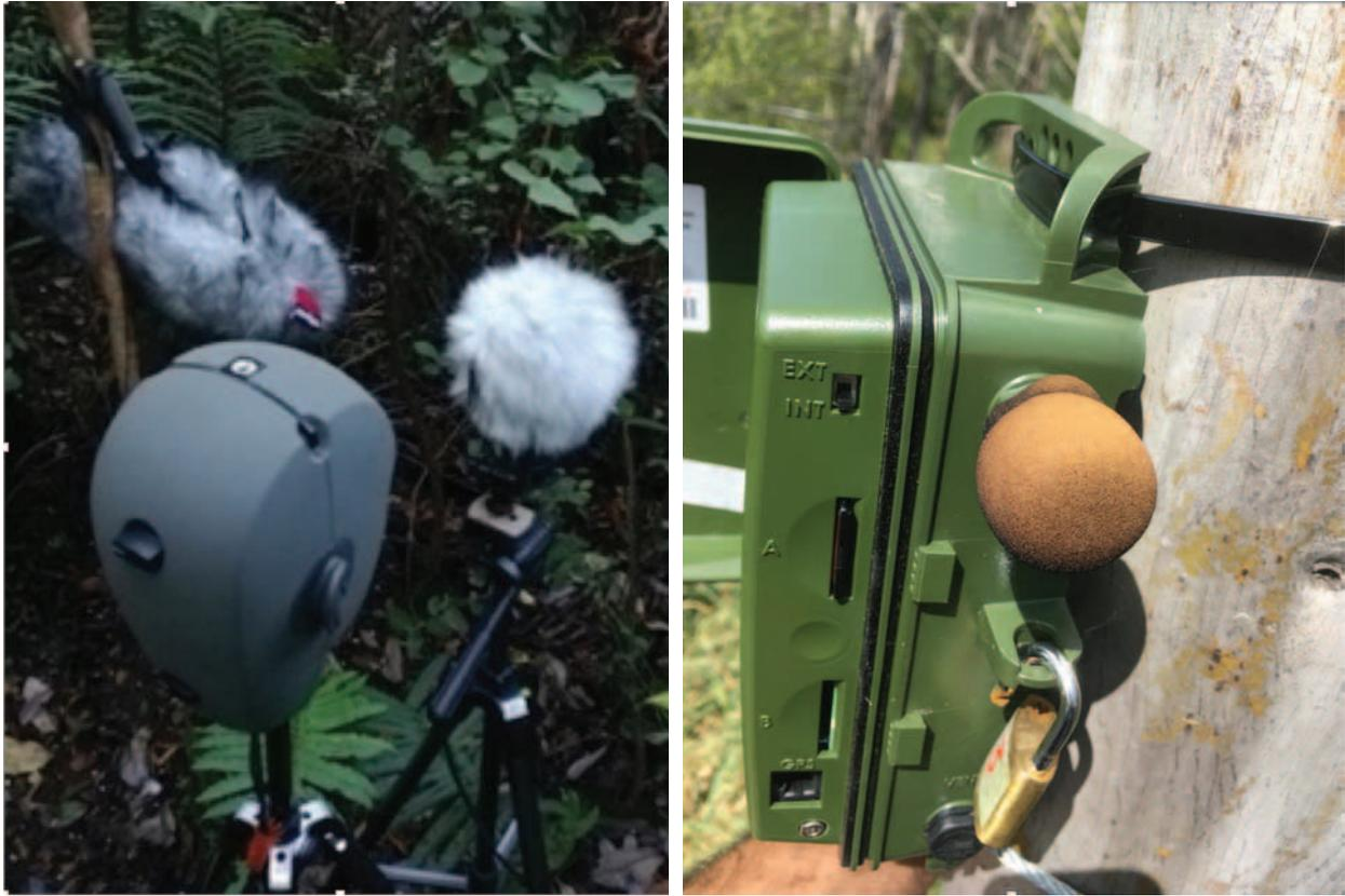
Field recording setups used to generate raw material for the time-lapse montage method. Stereo recording system for discrete recordings (left) and 8-channel microphone setup for continuous recordings in various spatial audio formats (right). (See the article in this issue by Felipe Otondo and André Rabello-Mestre. © Felipe Otondo.)
