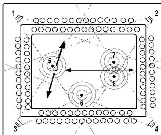
**Figure 1.** Setup for tests carried out at Lancaster University using an 8-channel mix played through a fixed quad system surrounding the audience and two pairs of commercial *Rimax* loudspeakers carried by two performers.
