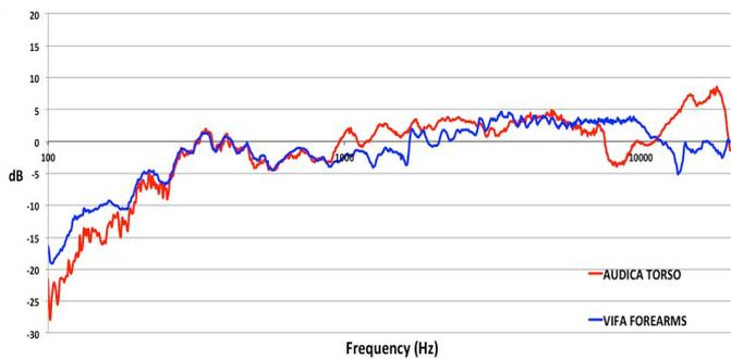
Figure 3: Frequency response of torso and arms’ loudspeakers.
