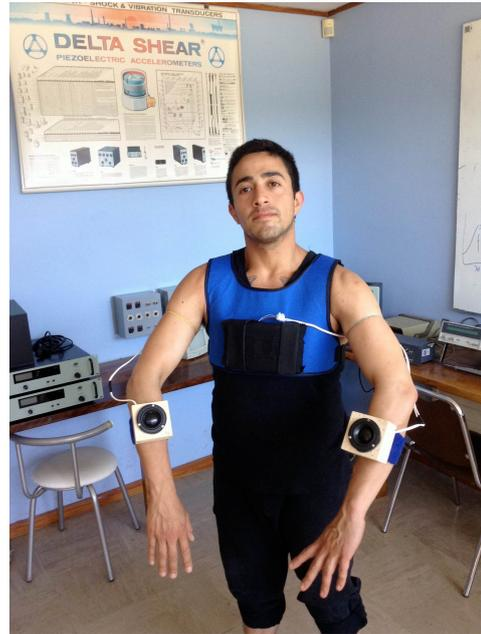
Figure 4. Dancer Ignacio Diaz testing the optimized body-worn system with one speaker on the torso and two speakers on the forearms.
