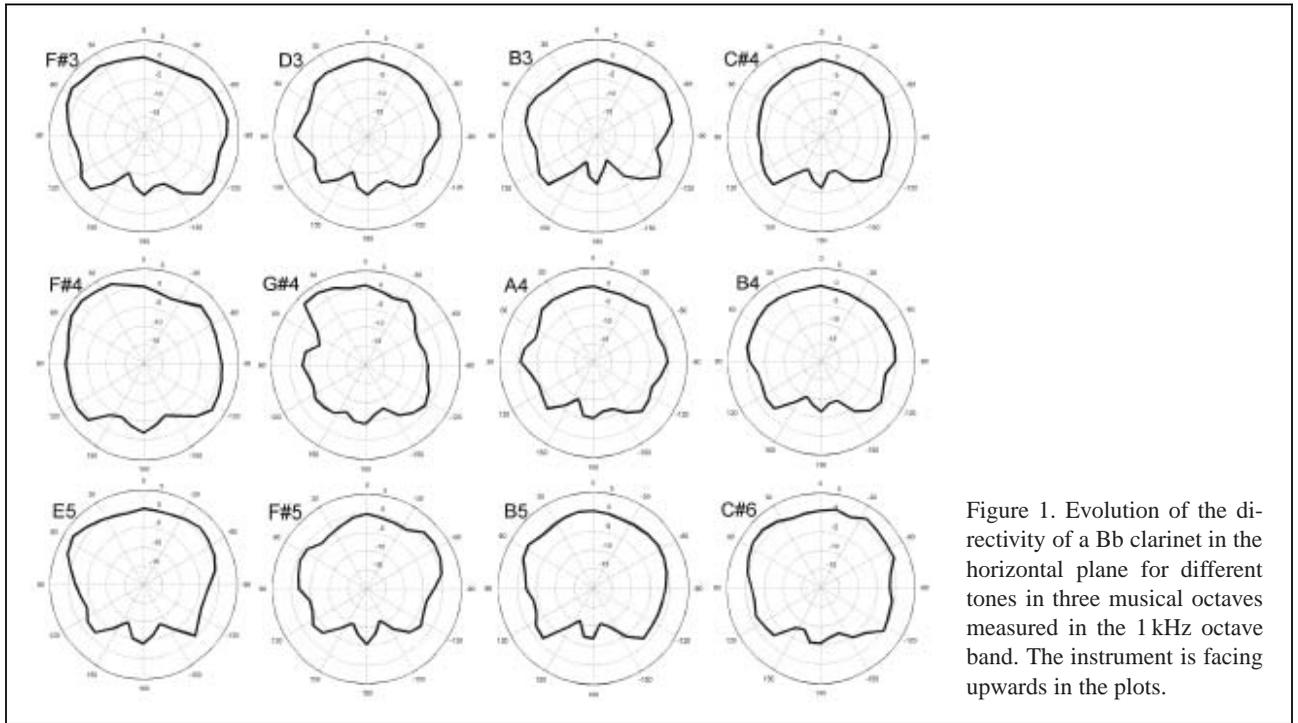
Figure 1. Evolution of the directivity of a Bb clarinet in the horizontal plane for different tones in three musical octaves measured in the 1 kHz octave band. The instrument is facing upwards in the plots.
