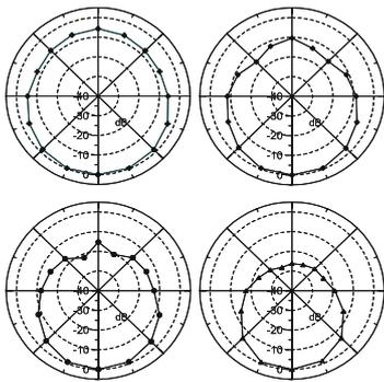
Figure 3: Measured directivity of the wood box loudspeaker in the horizontal and vertical plane at 500 Hz (above-left), 1000 Hz (above-right), 2000 Hz (below-left) and 4000 Hz (below-right) octave bands.
