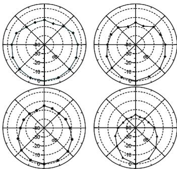
Figure 4: Measured directivity of the dodecahedron omnidirectional source with just one frontal unit turned on. Horizontal and vertical plane at 500 Hz (above-left), 1000 Hz (above-right), 2000 Hz (below-left) and 4000 Hz (below-right) octave bands.
