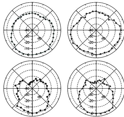
Figure 1: Measured directivity of the soprano singer in the horizontal plane at 500 Hz (above-left), 1000 Hz (above-right), 2000 Hz (below-left) and 4000 Hz (below-right) octave bands.
