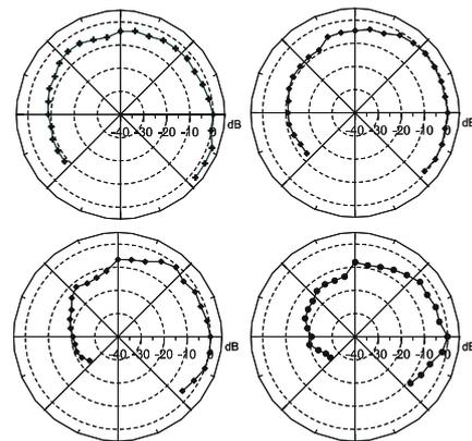
Figure 2: Measured directivity of the soprano singer in the vertical plane at 500 Hz (above-left), 1000 Hz (above-right), 2000 Hz (below-left) and 4000 Hz (below-right) octave bands.
