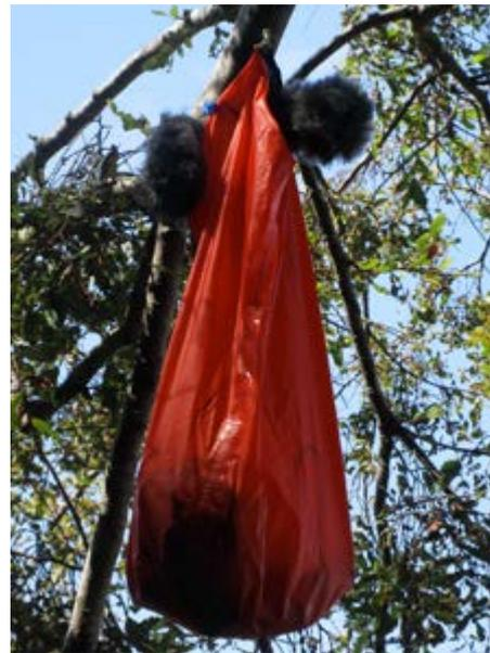
**Figure 2.** Field recordings setup designed for wetland with omnidirectional microphones hanging at the sides of a closed plastic bag.
