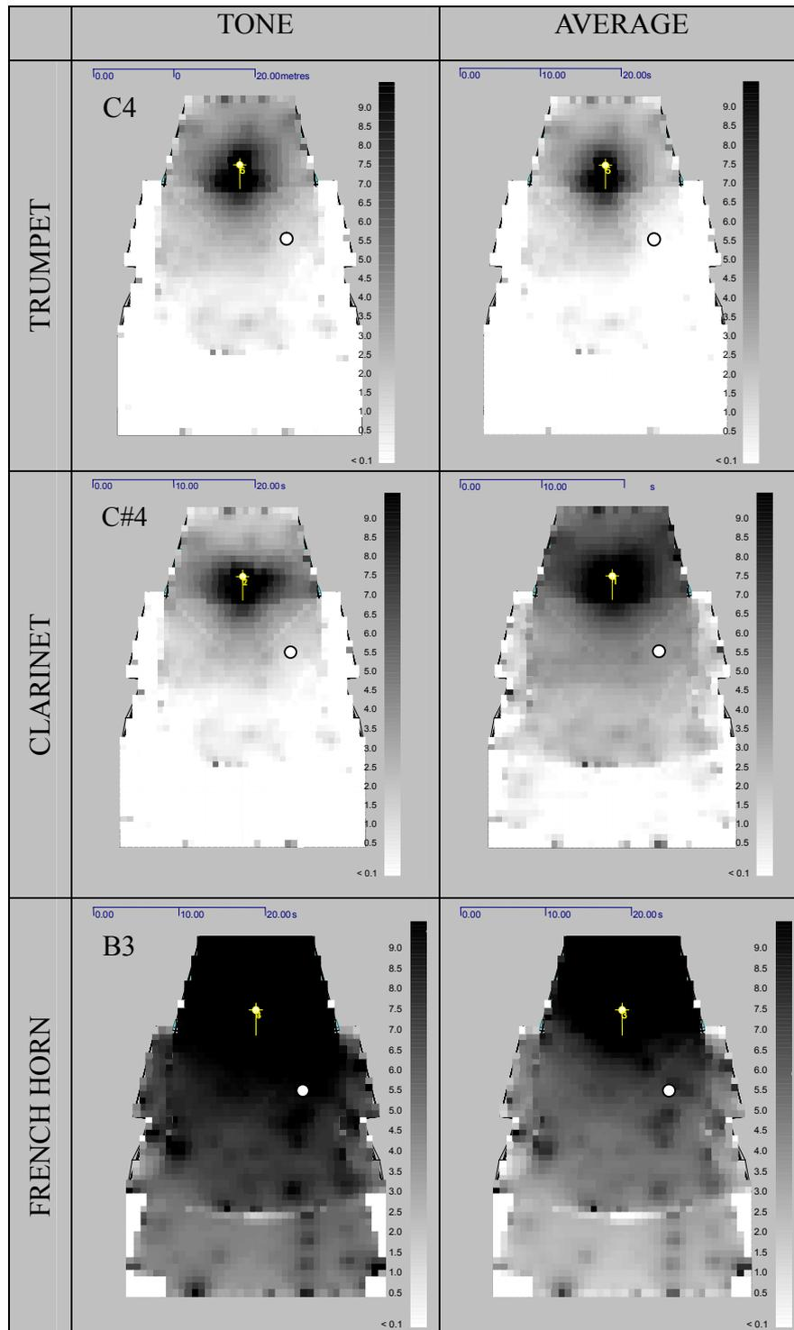
Fig. 3. Grid-response of the sound pressure level (SPL) of the three musical instruments in the 1 kHz octave band, simulated at the ELMIA concert hall with the directivity of a tone and the averaged directivity. The scale is relative and shown from 0 to 10 dB with white and black as the minimum and maximum values, respectively.
