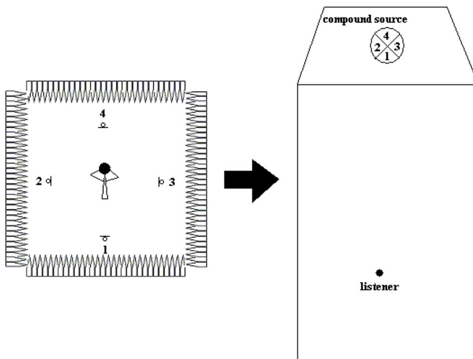
*Fig 4. The principle of the multi-channel method, here shown with four channels. Left: Anechoic recording of the source with four microphones, Right: Room simulation with the source represented by four directive partial sources.*
