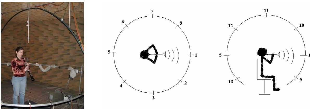
*Fig. 1. Left: A musician during the directivity measurements using 13 microphones with a radius of 1,5 m in the anechoic chamber. Middle: Microphone positions in the horizontal plane. Right: Microphone positions in the vertical plane.*
