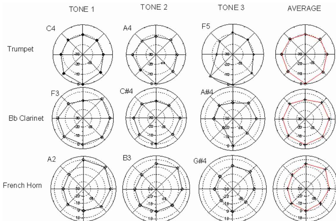
Fig. 2. Measured directivities for the trumpet, the clarinet, and the French horn for three different musical tones in the 1 kHz octave band in the horizontal axis. The front of the instruments is facing downwards. The averaged directivities in the right column correspond to the average over the whole pitch performing range of the instruments.
