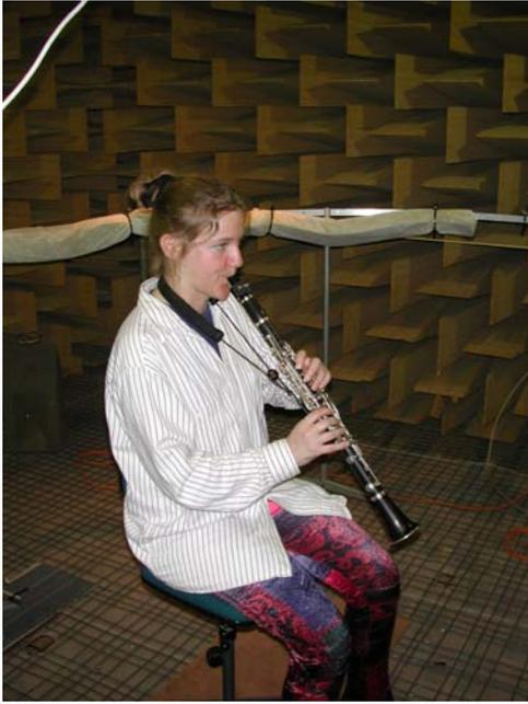
Fig. 1. Clarinet player during the directivity measurement in the anechoic chamber.
