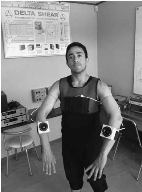
**Figure 7.** Dancer Ignacio Díaz testing the optimised wireless body-worn system with one speaker on the torso and two speakers on the forearms.
