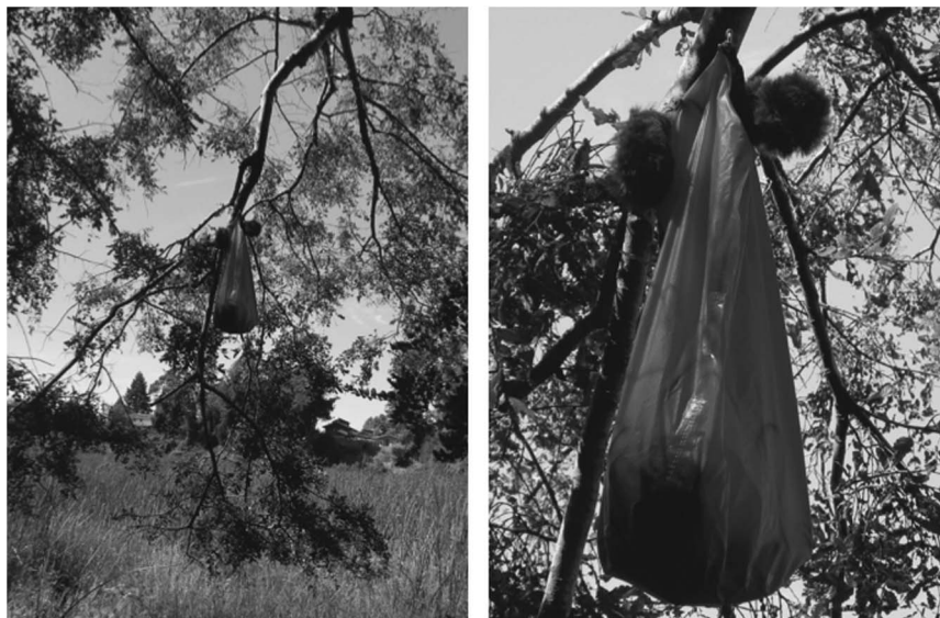
Figure 3. Recording setup used for recordings at the wetland in Valdivia, Chile. Left: stereo microphone array hanging from a tree at the side of the wetland. Right: close up of recording setup showing omnidirectional microphones with windjammer filters hanging at the sides of a hermetic plastic bag.
