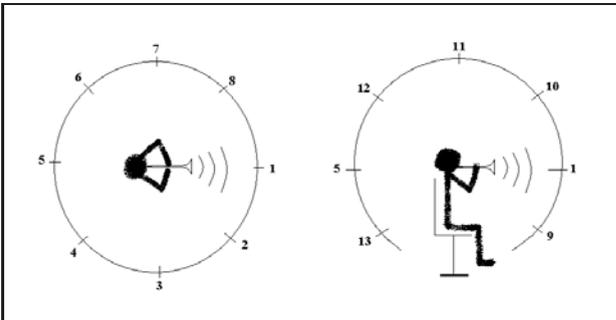
Figure 2. Setup for the simultaneous directivity measurements with 13 microphones. The left part of the figure shows the setup in the horizontal plane and the right part shows it in the vertical plane. Microphones 1 and 5 appear in both planes.
